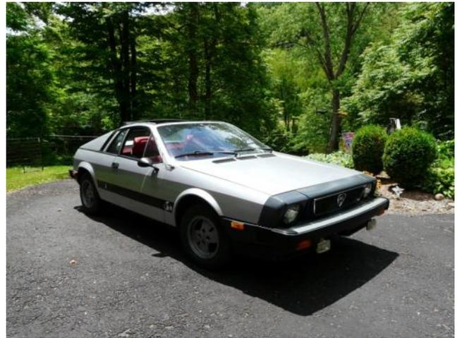
level of equipment, Lancia chose a two-litre twin-cam four-cylinder motor from Fiat 124 Sport Coupe, MacPherson suspension, five-speed gearbox, and 4 wheel disc brakes. Total production of the Montecarlo in Europe came to 7798.
